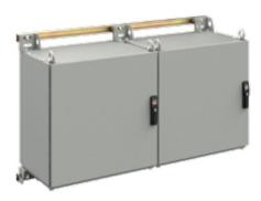
The PROLINE G2 Anti-Tip Bracket Kit secures the top of an enclosure to a fixed surface such as a wall, and protects against enclosure tipping. The brackets are made from 10 gauge mild steel, and are Polyester powder-painted RAL 7035 textured light gray. The kit comes with a single pair of brackets and mounting hardware to affix brackets to the enclosure.
